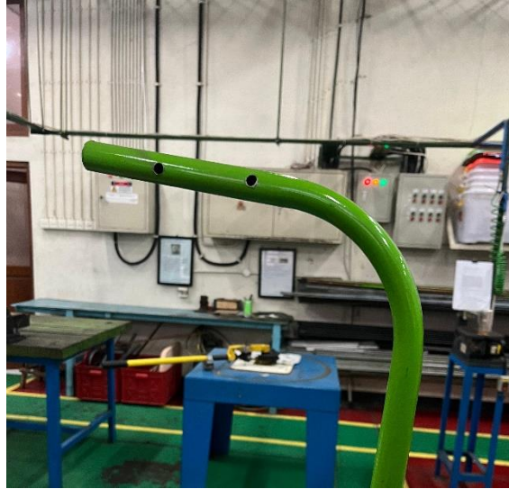
Gambar 2. Hasil Drilling Tanpa Jig
