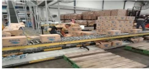
Gambar 1. Proses *Manual Palletizing*
