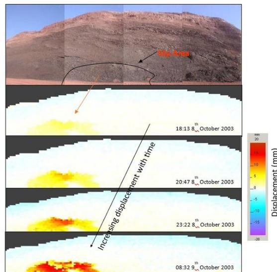
Gambar 2. SSR Output Data – Deformation (Harries & Cabrejo 2010)
